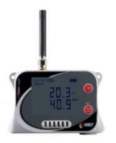
GSM datalogger is designed to record temperature and humidity humidity. In case of exceeded set limits, SMS and JSON messages can be sent via GPRS data connection. It is possible to set the regular sending of JSON messages to Comet Database, the sending interval is adjustable. The recording is performed in a non-volatile electronic memory. The data can be transferred to a PC via USB-C.
